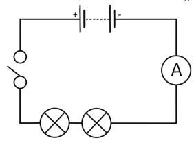
3. Draw a series circuit with 1 cell, 2 bulbs and a closed switch.
