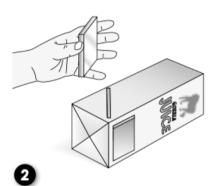
From the bottom of each carton, measure a 45° angle and cut a slot on both sides of the carton. The slot should be big enough to fit a mirror into the slot.
