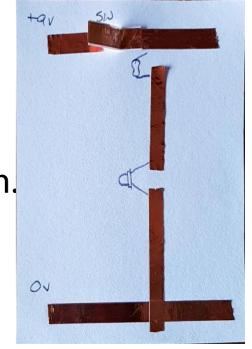
• All joints need to be tinned first. Then components are added
