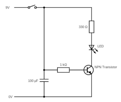
Draw the circuit using Tinkercad circuits and then assemble on your breadboard. When done... Use the copper tape, components and soldering to make it.
