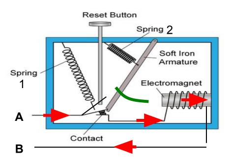
Current normally flows between terminals **A** and **B** through the contact and the electromagnet.
