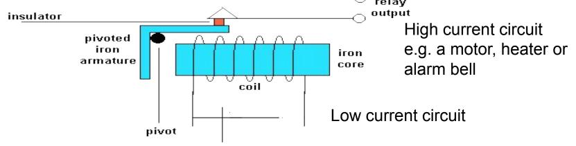
• When the switch is close, current flows to the electromagnet which
