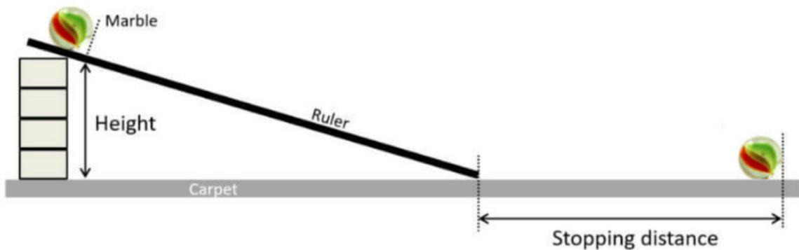
1. Set up the equipment as shown in the diagram.
