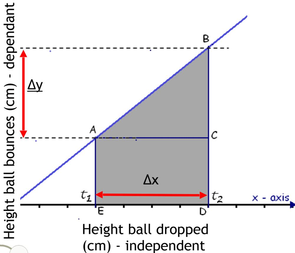
A line graph can be used to calculate gradient. The co-ordinates of a straight line in the graph are taken (for example from A to B) by projecting back to the x and y axis.
