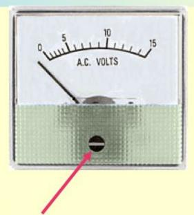
Use a screwdriver here to adjust the pointer.
