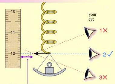
It is due to the gap here, between the pointer and the scale.
