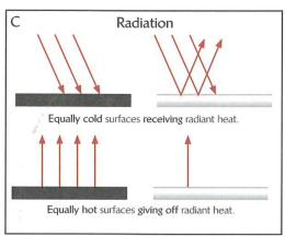
Can send heat through still air or empty space. This drawing shows the importance of colour in absorbing and giving off IR (infrared) heat. Texture is also important: shiny surfaces absorb and give off least heat, while matt (rough) surfaces absorb and give off most heat.
