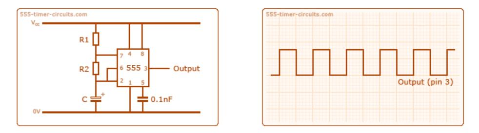
• This type of circuit could be used to give a mechanism intermittent motion by switching a motor on and off at regular intervals. It can also be used to flash lamps and LEDs, and is useful as a 'clock' pulse for other digital ICs and circuits.
