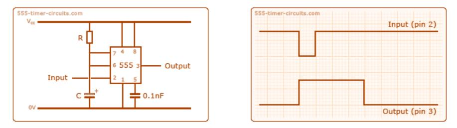
This type of circuit is ideal for use in a "push to operate" system for a model displayed at exhibitions. A visitor can push a button to start a model's mechanism moving, and the mechanism will automatically switch off after a set time.
