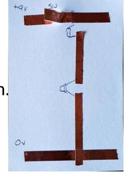
• All joints need to be tinned first. Then components are added
