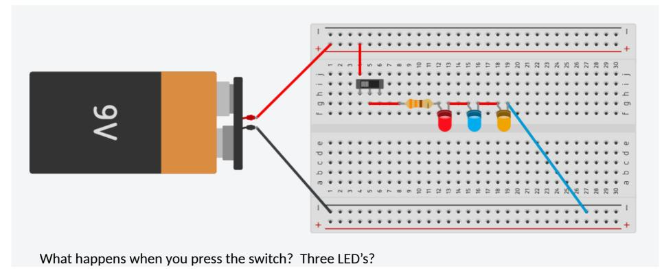
Measure the voltage across the resistor and each of the LED's
