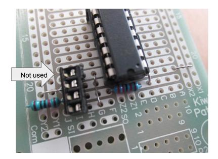
This view shows the picaxe 14M2 with its download connections and also its +ve and -ve connections to the outer rails on the circuit board, check by looking at the example circuit board to make sure you get all the links in the correct places.
