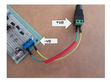
This photo shows the completed circuit board with the 12 volt power supply socket. The positive wire has the piece of red shrink tube to identify it as the hook-up wires are multi coloured.
