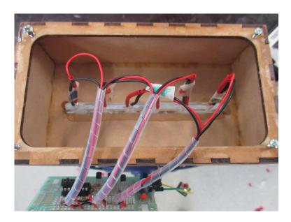
The led's are inserted into the edge of the acrylic plate in the order of green, red, blue, green, red, blue. The led's must be fully pushed into the holes
