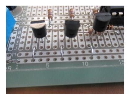
This photo shows the transistors. Each transistor has a connector link between its emitter lead and the negative rail. The link wire at the bottom left of the photo is connecting the negative rail to the negative of the power supply block (blue)
