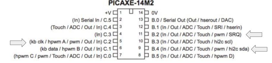
The picaxe 14M2 microcontroller. The three output pins used are c.2. b.4 and b.2
