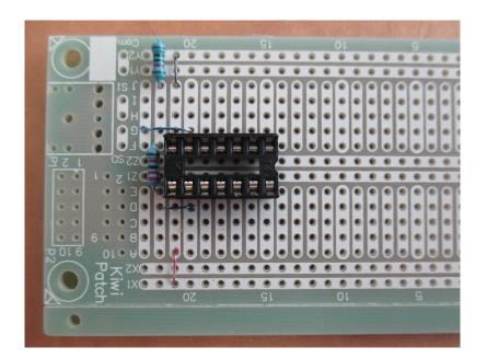
Insert the 14 pin insert, 22k resistor above the insert and the 10K resistor in the same row to -ve. The other wire connectors are:
