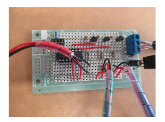
The completed circuit board with the 6 led's inserted. The led's must be in pairs, red, green and blue, the photo shows the colours marked on the coils around each pair of led's The negative leads connect to the 180 ohm resistors which you can see int he centre of the
