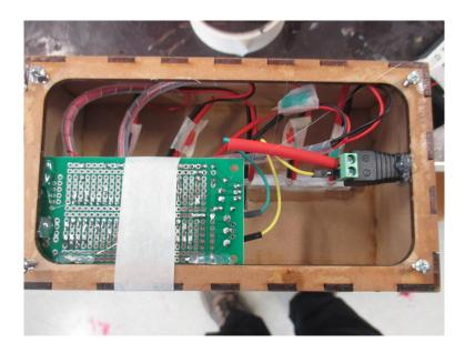
This photo shows the circuit board and the 12 volt power socket inserted into the case.
