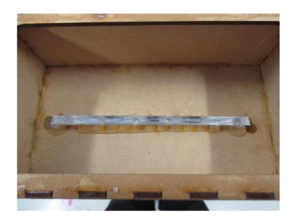
When the position of the plate has been checked, fully glue the plate by running hot glue along each side of the plate to the case.
