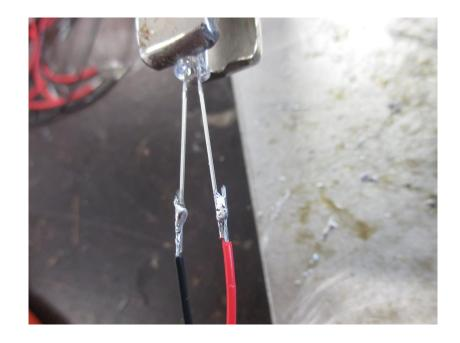
Solder each wire to the led leads, there is no need to add solder, just hold the 10mm end of the wire parallel with the lead running the tip of the iron slowly along the joint.
