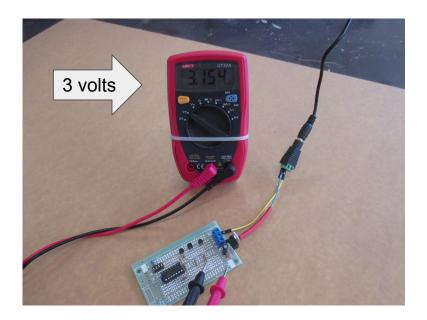
Next, check the voltage between the 3 x 180 ohm resistors which are connected to the transistor collector leads. Place the -ve lead on the resistor lead and the +ve lead on the connector wire that connects the power supply to the +ve rail, the multimeter should show around 3 volts, which is the correct voltage that the two led's need to run
