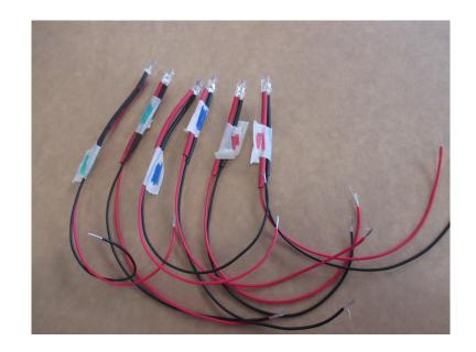
Make six led's (2 x green 2 x red and 2 x blue) the wire must be stranded/flexible type
