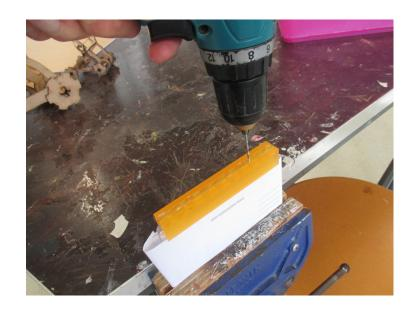
Secure the acrylic using a vice to hold it firmly. Place a hole drilling jig on the bottom edge of the acrylic, this will be used to mark the six equally spaced 5mm holes which will hold the led's, a piece of tape can be used to hold the jig in the centre.
