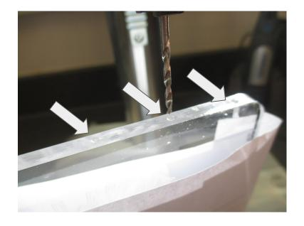
Secure a 2mm drill bit into the machine drill. Hold the acrylic firmly in the machine vice, the edge should be horizontal and level
