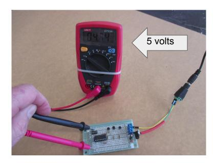
When the power supply and picaxe have been soldered you MUST check that you have the correct voltage supplied to the circuit board.
