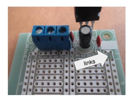
The voltage regulator leads are pushed through the circuit board only 1 - 2 mm for soldering.
