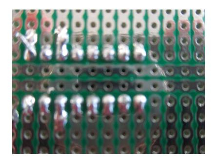
Solder joints must be absolutely perfect, the solder completely around the lead, smooth and shiny, no cross connections
