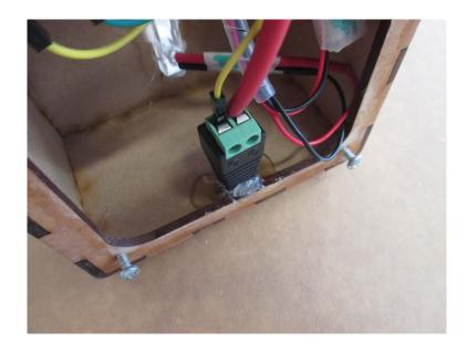
After drilling an 8mm hole in the case side, glue in place the 12 volt power socket. A small blob is used on the edge of the case to hold it in place then check the position is OK before adding glue inside the case each side of the socket.
