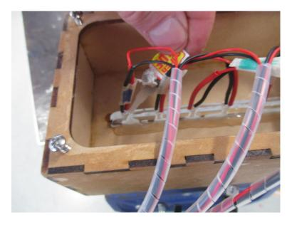
Add a drop of super glue to the top of each led where it meets the acrylic and let it set for 5 minutes. Be very careful when using super glue, it will instantly glue skin together and should not come into contact with skin, eyes and clothes. If it contacts your skin then Acetone is the only chemical that will melt it, your teacher will deal with this.
