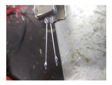
Add a spot of solder to the end of each led lead
