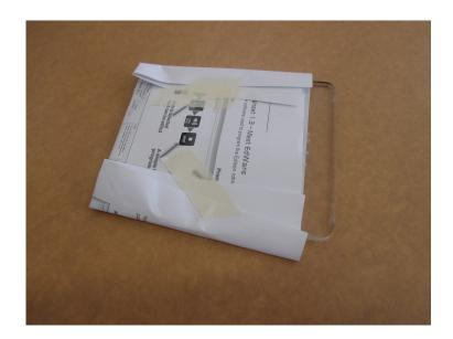
After the moodlight has been laser cut and engraved wrap the piece of acrylic in a sheet of paper folded to fit the size, this will prevent scratches and marks on the surfaces during the assembly process.
