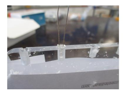
The 5mm holes should be drilled just deep enough so that an led fits flush with the edge of the acrylic, the machine drill can be set so that it drills to a specific depth.
