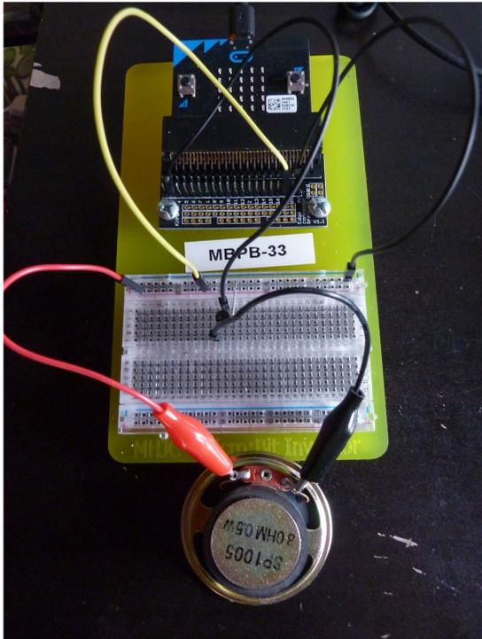
This photo shows all of the connections between the speaker, bread board and Micro:bit edge board
