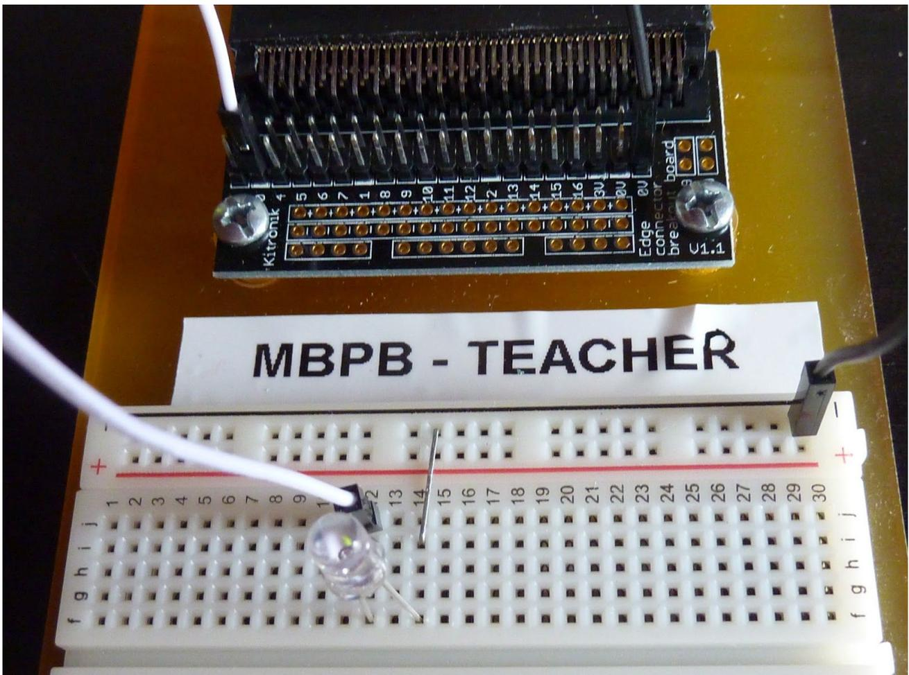
We will use the prototype board to build a series of circuits using electronic components such as Light Emitting Diodes (LED's) and Light Dependant Resistors (LDR's) along with jumper wires, jumper wires can also be made by using ordinary paper staples.
