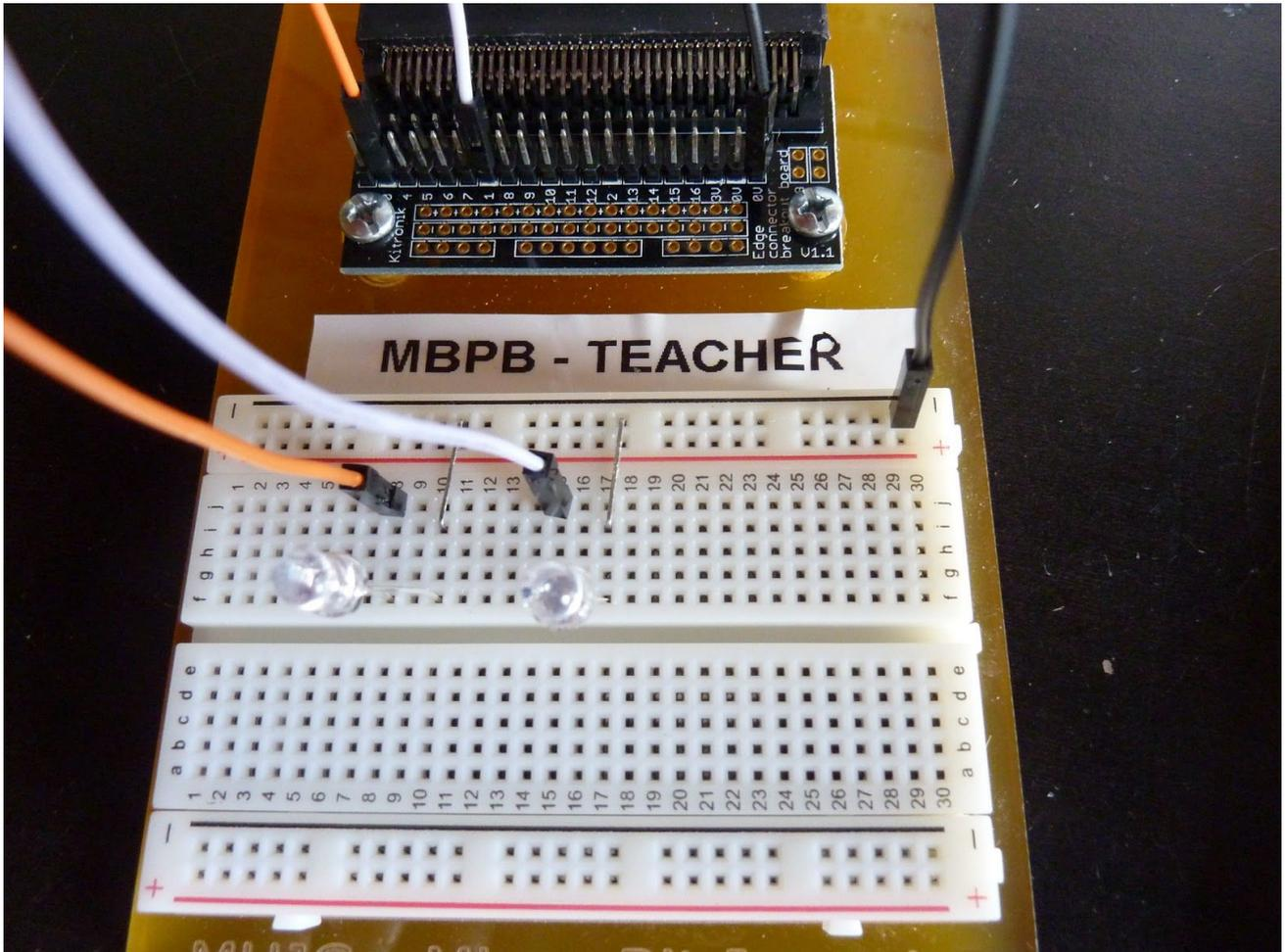
This photo shows the breadboard connections for experiment #2 - 2 x led's, green led on the left, red led on the right.
