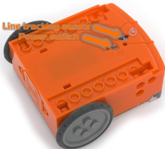
Edison's power switch and line tracking sensor
